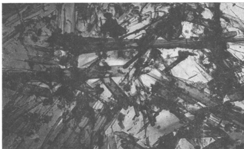
Fig. 2. Microstructure of gypsum stone obtained by standard curing.
